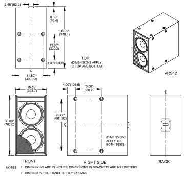
3. SYMBOL () INDICATES MOUNTING POINT, 3/8 INCH-16 THREADED HOLE (PI ANGLE)
